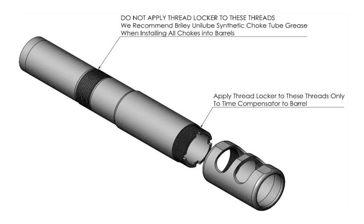
Note: We recommend using Loctite 271 High Strength or similar when timing the compensator. When the compensators are timed they will be specific to the barrel they were timed in. However, if you have multiple guns and might switch the chokes between them, Loctite 242 or similar can be used to allow for easier retiming of the compensator.
